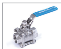
3- Piece Ball Valve 31K TYPE 1/4" – 4" INVESTMENT CASTING BODY & CAP / ASTM A 351 - CF8M (DIN 1.4408) / ASTM A 351 – CF8 (DIN 1.4301) ASTM A 216 – WCB (DIN 1.0619)
