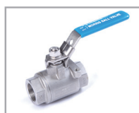
2- Piece Ball Valve 22K TYPE 1/4" – 2" INVESTMENT CASTING BODY & CAP ASTM A 351 - CF8M / ASTM A 351 – CF8 / ASTM A 216 - WCB
