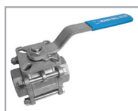
3- Piece Ball Valve 31KM TYPE 1/4" – 4" ASTM A 351 - CF8M (DIN 1.4408) / ASTM A 351 – CF8 (DIN 1.4301) ASTM A 216 – WCB (DIN 1.0619)
